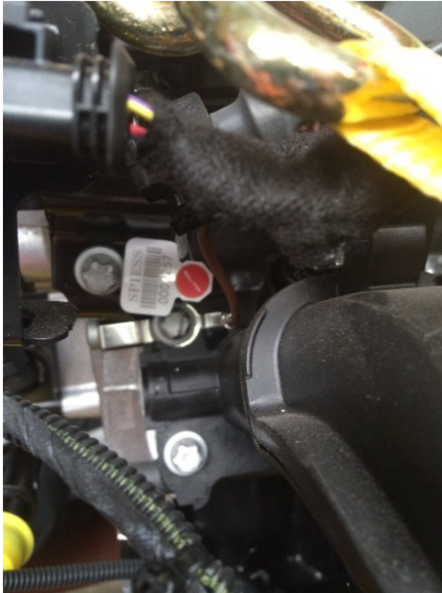
Bild 4 (Plombe 1 ZSB Motor – Zylinderkopf): Picture 4 (Seal 1 engine assembly – cylinder head):
